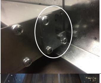
Using a T27 torx bit, remove the 3 outer screws from the end of the 2 x extrusions inside the drawer.
