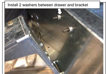
Note that the installation of the SBRK-1 will be different when installing the RDK.
