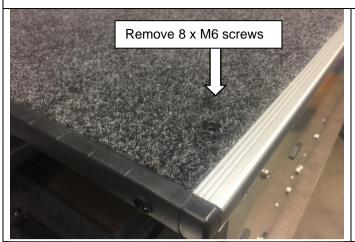
Using a 4mm allen key remove the 8 x M6 countersunk screws securing the top carpet panel to the drawer.
