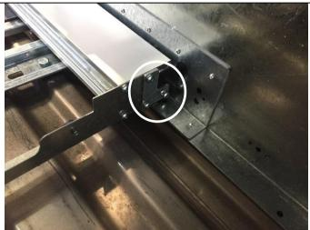
Re-install the inner and outer trolley assembly to the cabinet.
